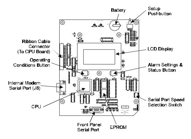
Figure 2-7: CPU Circuit Board
